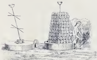
№7. STEAMING CLOTHS DURING THE PROCESS OF BLEACHING
