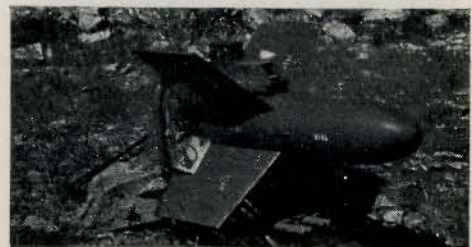
Nord S.S.10 wire guided solid fuel anti-tank missile. 80% accurate over 1 mile range. Launched from ground or aircraft. Weight 35 lb.
