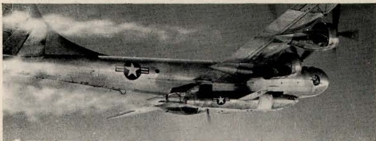
Bell X-1A research aircraft being carried to its launching height under an EB-29 Superfortress mother-plane. The X-1A has reached a height of 90,000 ft. and speed of 1,650 m.p.h.
