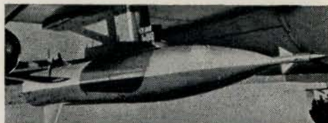
Matra O51 2-stage solid fuel air to air guided missile. Supersonic. Proximity head. Weight 350 lb. Length 10 ft.
