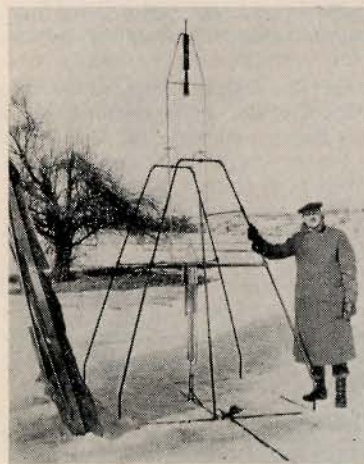
This spidery contraption was Goddard's first successful liquid propellant rocket, fired on 16th March 1926.
