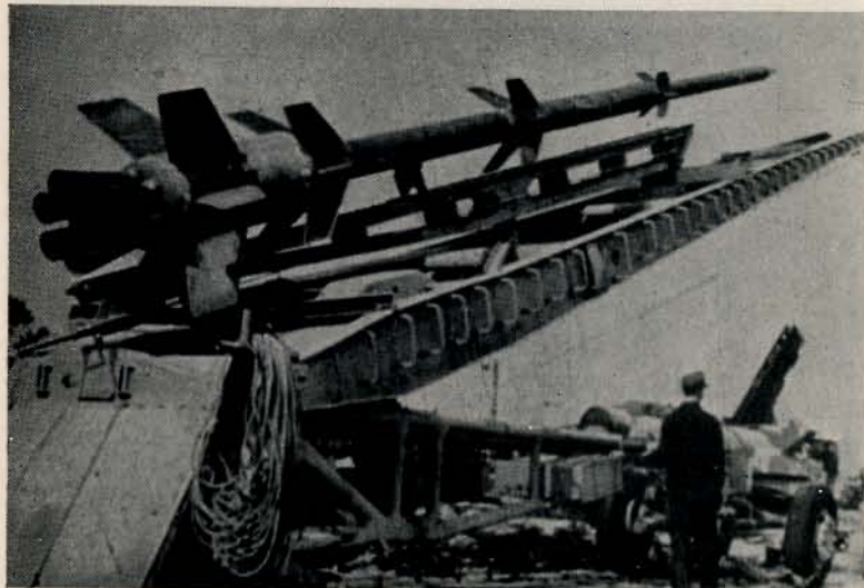
The German Rheinbote four-stage rocket was fired operationally against Antwerp in World War II. Take-off weight was 1.7 tons and the third step, which carried an 88-lb. warhead, achieved a speed of 3,600 m.p.h. and range of 140 miles.
